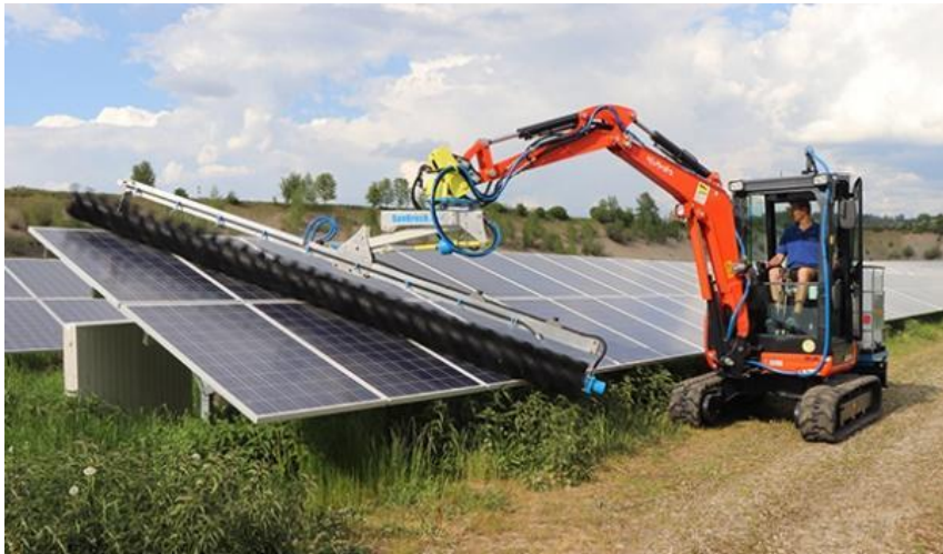
Figure 8: Solar cleaning system. Image source: www.sunbrushmobil.com
